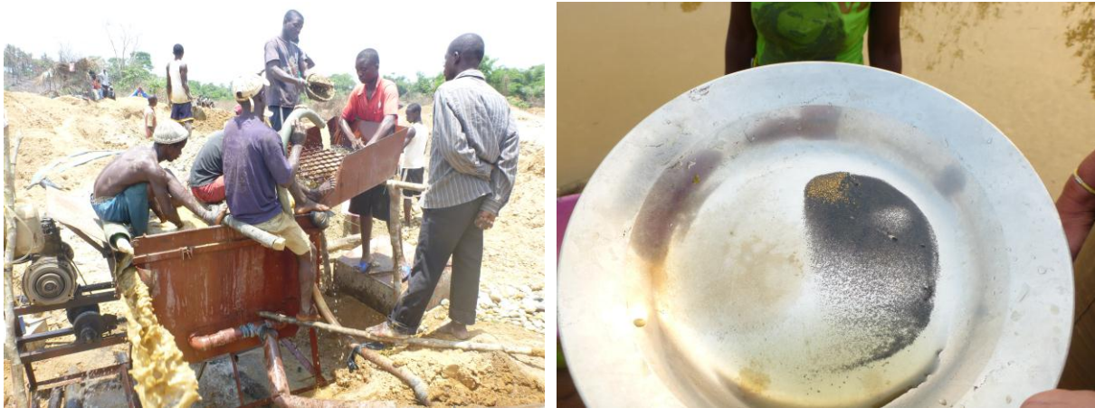
Using a mechanical jig to process the gold and diamond bearing gravel – gold recovered from sluice box
